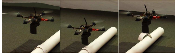
Figure 2.19: images from a sample “swooping” trajectory using the vision-based controller developed in this paper.
